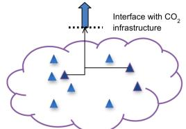
Overview of a cluster with CO<sub>2</sub> sources, the collection network and the system boundary with long-distance transport
