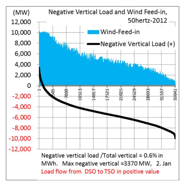
When wind feed-in was very high, negative vertical load happened. Excess wind feed-in was transferred from DSO grid to TSO grid. Source: Calculated by 50hertz's grid data Kennzahlen in 2011 and 2012
