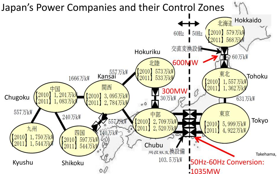
万kW = 10MW. Nine circles show each major power company's control zone. Figures in each circle show maximum electricity demand in each control zone. Figures between circles: Capacity of main transmission lines between control zones.
